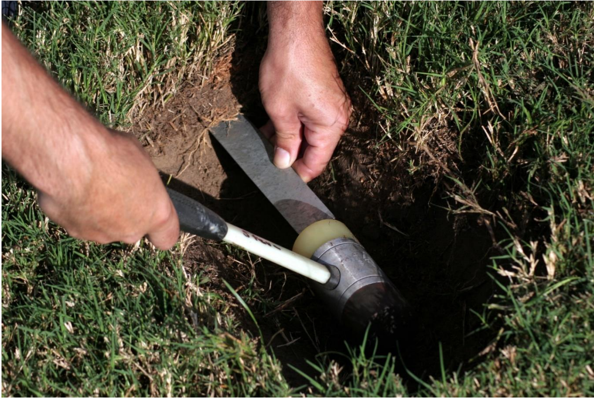
Figure 11. Root cutting procedure preparing soil for SMS installation
