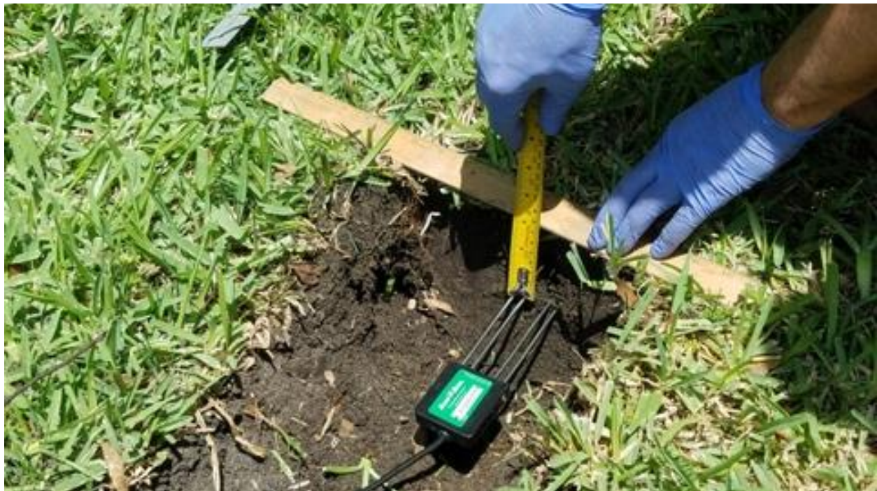
Figure 12. Depth recommended to insert the probes (3 inches deep)
