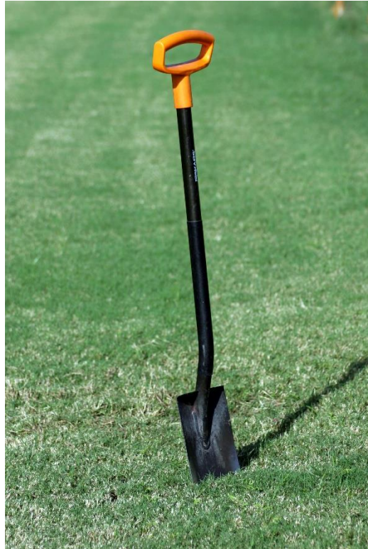
Figure 8. Square-point ditching shovel required for SMS installation
