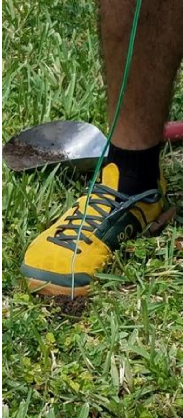
Figure 21. Packing native soil around the probe
