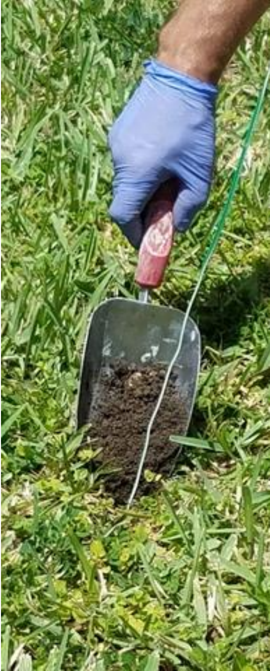
Figure 21. Packing native soil around the probe
