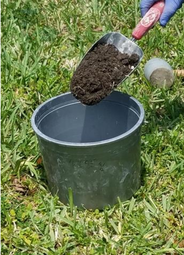
Figure 18. Mixing a slurry of native soil and water
