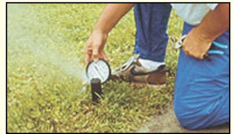
PERFORMING A PRESSURE GAUGE TEST
